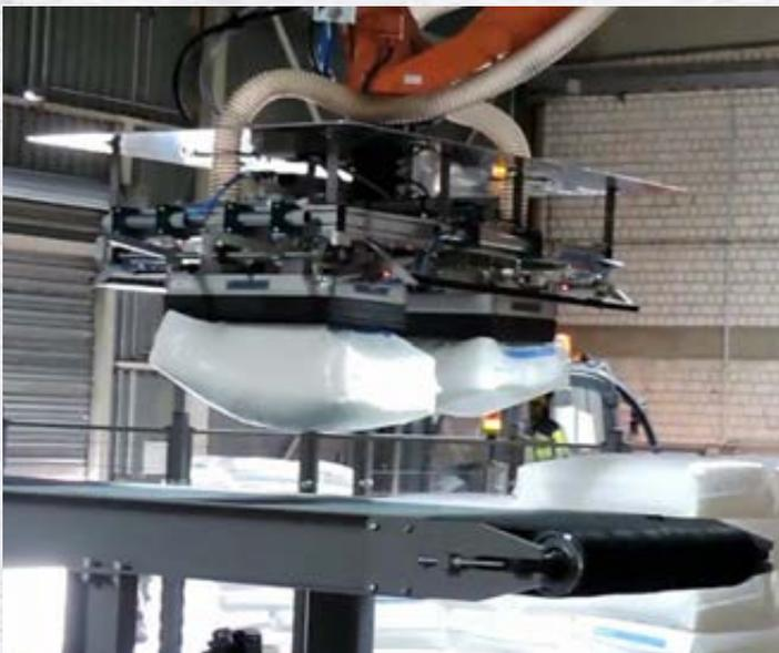
The UniGripper BagGripper comprises customized grippers for bags, pouches and similar products of almost any size. Most commonly the BagGripper is delivered with a side channel blower, efficiently providing high vacuum flows and the ability to handle very loose bags where alternative solutions often fail.
