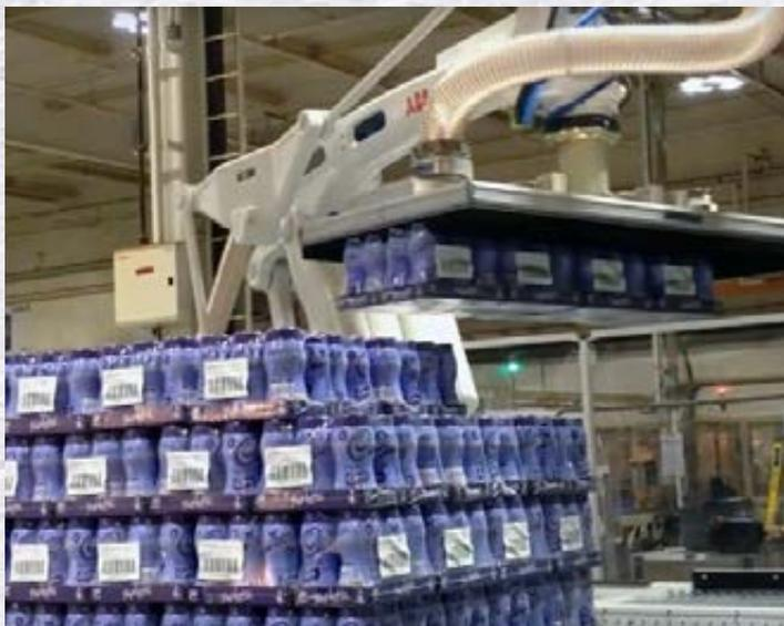
Palletizing of boxes, trays and shrink wraps can be enabled with the same UniGripper. Depending on product properties as well as what is most optimal for each installation, the vacuum source can either be venturi ejectors or a side channel blower.
