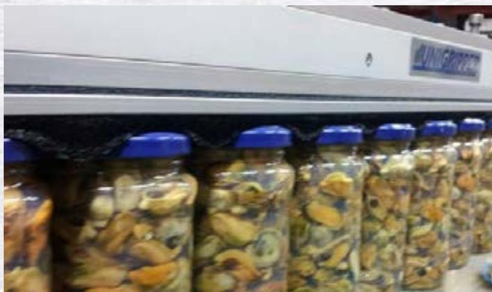
UniGrippers for jars and cans provides the ability to handle large variations of open or closed containers. The intelligent vacuum technique allows a single gripper to handle various sizes without any kind of modification of the gripper head.
